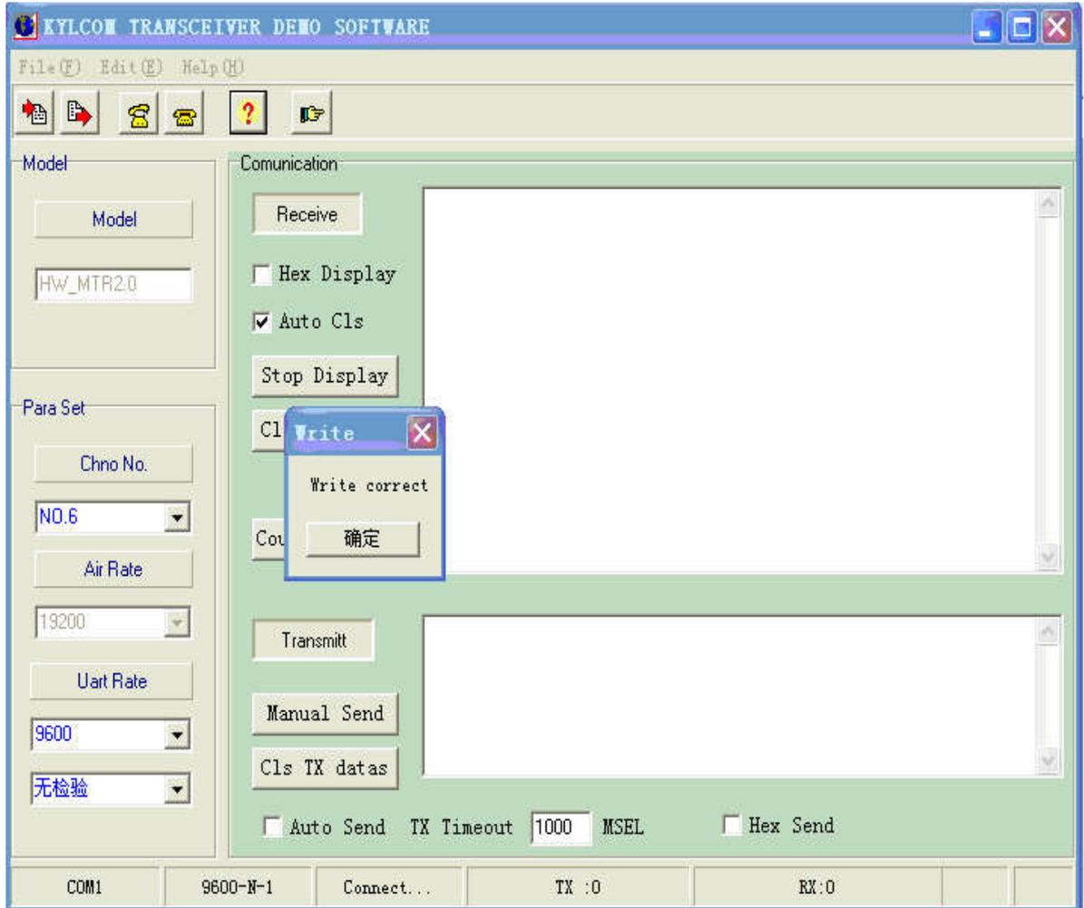
**Note: The RF data rate(Air Rate) can not be set by user, it is confirmed when placing orders and set before delivery. So please confirm the RF data rate when placing the order.**
