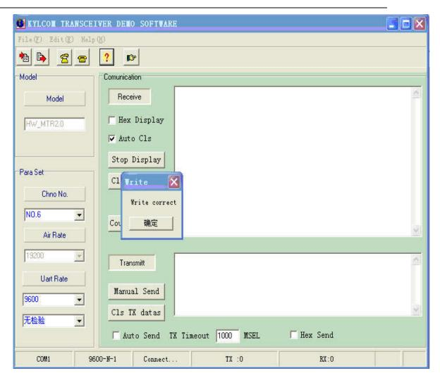
Note: The RF data rate(Air Rate) can not be set by user, it is confirmed when placing orders and set before delivery. So please confirm the RF data rate when placing the order.
